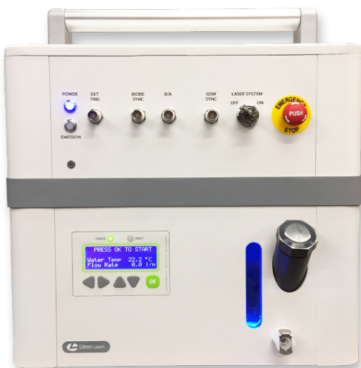
Free standing PSU and chiller (separate units)
